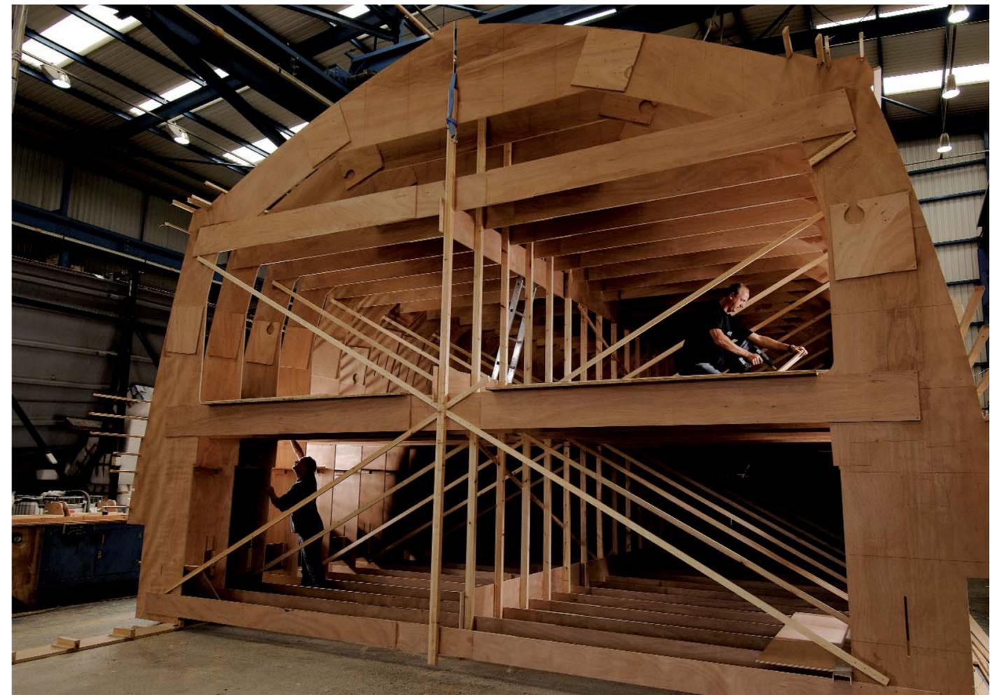
Hand-building the timber plug – the basis of all large-hull Sunseeker models.
